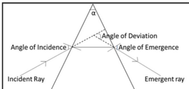
Figure 2: Optics of a prism
