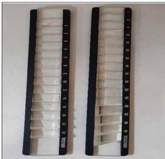
Figure 7: Prism bars with vertical and horizontal prisms
