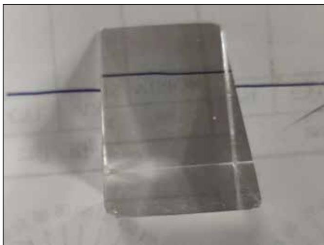
Figure 3: A straight line drawn on a paper appears displaced towards the apex of the prism
