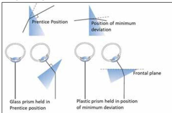
Figure 4: Positioning of prisms
