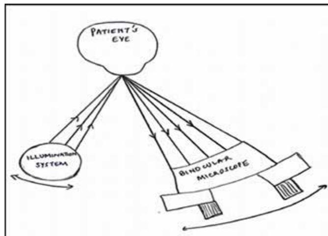
**Figure 1:** J. Slit lamp design includes binocular microscope & illumination system
