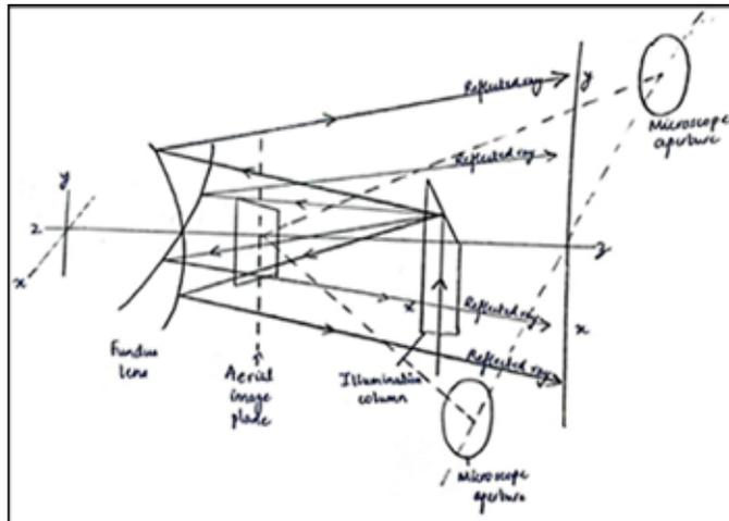
Figure 2: . Schematic representation of slit lamp apparatus
