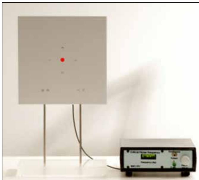
Figure 6: CFF Apparatus<sup>18</sup>
