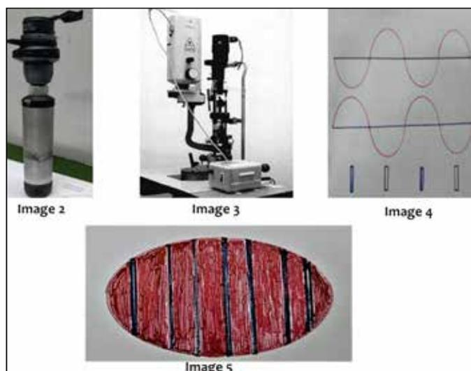
Figure 2,3,4,5: (2) Handheld LI (3) Slit-lamp mounted LI (4) Coherent light beams (5) Diagrammatic representation of Interference Fringes
